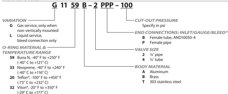
If bleed connection is desired, add letter "P" for female pipe or "B" for female tube. Example: 1159B-2PPP-100 or 1159A-4BBB-100
