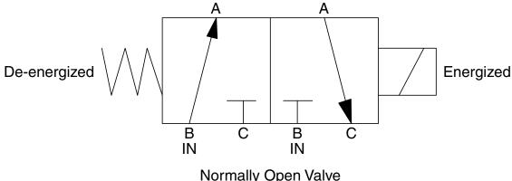
Normally Open Valve Port B is the inlet
