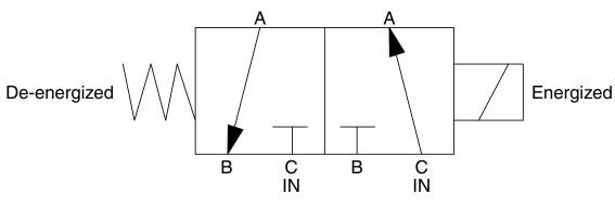
Normally Closed Valve Port C is the inlet
