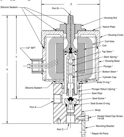
13230 1/2" 3-way valve, shown with a combination explosionproof NEMA 7 and waterproof NEMA 4 coil housing
