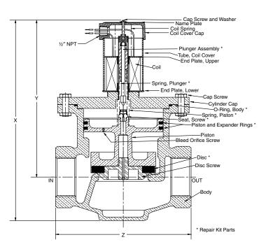
Normally open 2 ½" 5801 valve, shown with a NEMA 1 coil housing and a metal pilot seat
