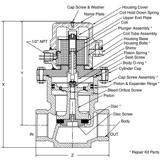
Normally closed 2" 5700 Valve, shown with a NEMA 7 explosion-proof coil housing and a soft pilot seat)
