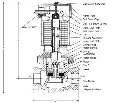
Normally closed 1" 4408 valve, shown with a NEMA 1 coil housing and a metal pilot seat
